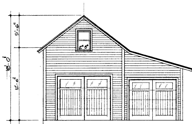
GARAGE - SOUTH ELEVATION SCALE: 1/4" = 1'-0" (REAR SIMILAR)
